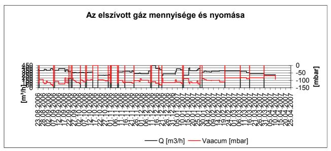
Diagram 1: Accompanying test evaluations, here: amount of gas and gas suction pressure
