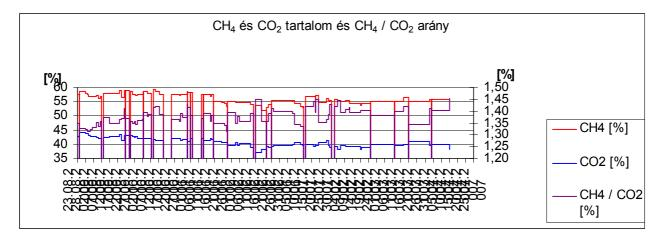
Diagram 2: Accompanying test evaluations, here: CH<sub>4</sub> and CO<sub>2</sub> – content in the row gas
